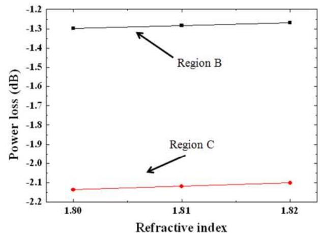
Fig 3. Propagation losses in PLCs as a function of refractive indices of SnO<sub>2</sub> thin films.
