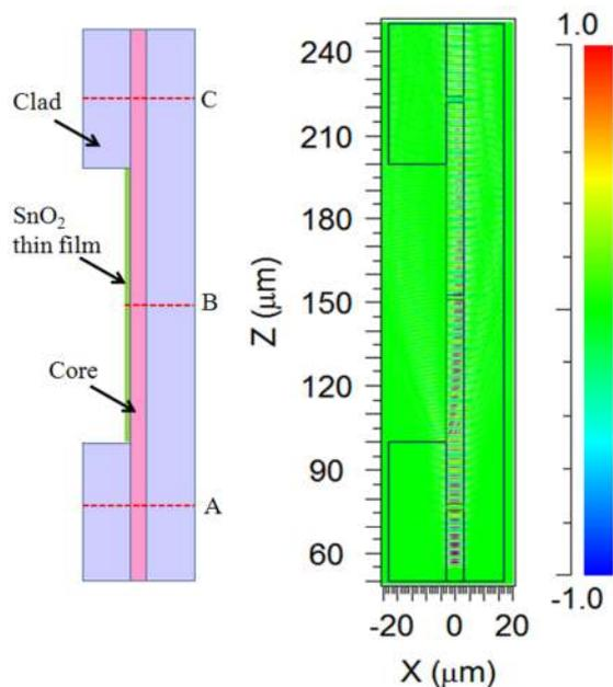
Fig 2. Propagation field intensity profiles in the PLC.
