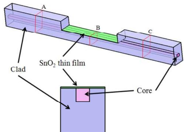
Fig 1. Schematic view of the PLC with SnO<sub>2</sub> thin film.
