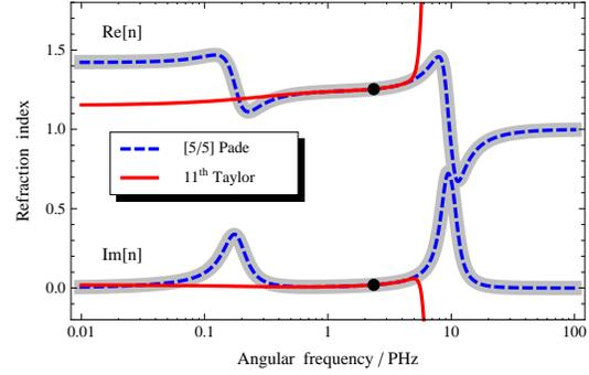
Fig. 4. Complex dispersion for the same material as in Fig. 1 (fat grey). Red: Taylor expansion (11th order), blue: [5/5] Pade approximation [8].
