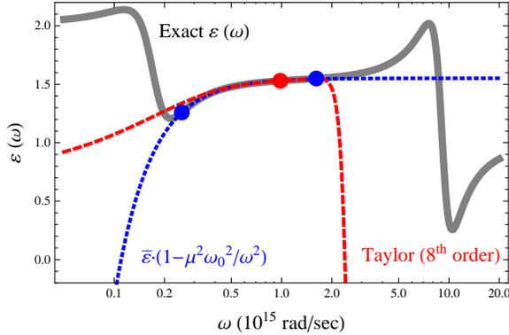
Fig. 3. Material response dispersion of fluoride glass (fat grey line) and a simple rational approximation to it (blue dashed line). For comparison also Taylor expansion of 8th order (red dashed line) is shown [3].
