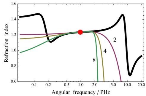
Fig. 1. Refractive index of fluoride glass (fat black line) and truncations of the Taylor expansion (color lines) of the order 2 (like in NSE), 4 and 8. Increase of the approximation order cannot resolve the divergence.
