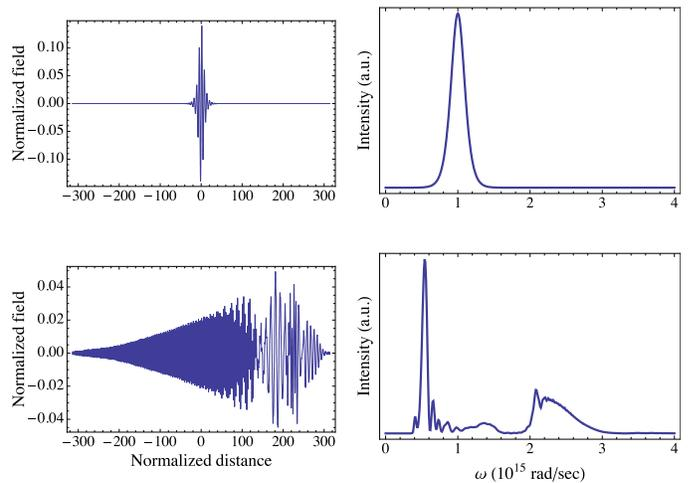
Fig. 2. Top: electric field (left) and spectrum (right) of the initial pulse. Bottom: the same after 10 ps propagation in a bulk Kerr medium with the refractive index shown in Fig. 1. The nonlinear susceptibility parameter  $\chi^{(3)}$  is used to normalize the fields.
