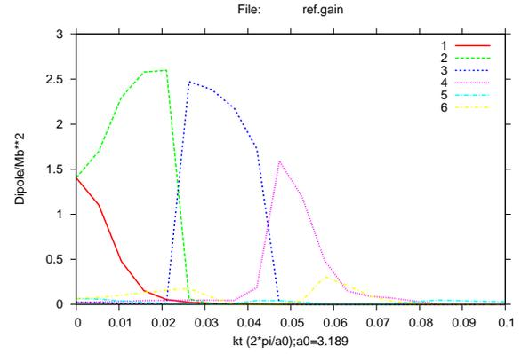
FIG. 3: Dipole transition from valence subbands to the conduction band for growth-plane (0001).
