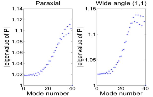
Fig. 2. Dependence of the magnitude of the eigenvalues of  $P$  on the mode number for the paraxial and wide angle scheme,  $\Delta x = 1 \mu\text{m}$  while  $\Delta z = -0.1 \mu\text{m}$ .
