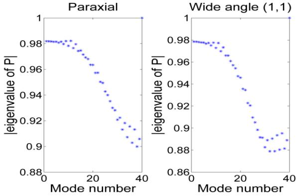
Fig. 1. Dependence of the magnitude of the eigenvalues of  $P$  on the mode number for the paraxial and wide angle scheme,  $\Delta x = 1 \mu\text{m}$  while  $\Delta z = 0.1 \mu\text{m}$ .
