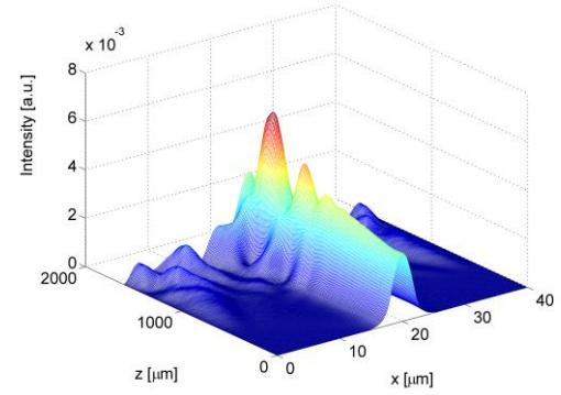
Fig. 3. Intensity distribution calculated by backpropagating the fundamental mode using C-N FD-BPM within 1600  $\mu\text{m}$  long waveguide,  $\Delta x = 0.1 \mu\text{m}$  while  $\Delta z = -0.1 \mu\text{m}$ .
