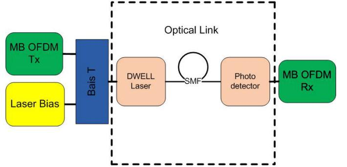
Fig. 1. Block diagram of the analogous optical link containing QD in the well (QDWELL) laser
