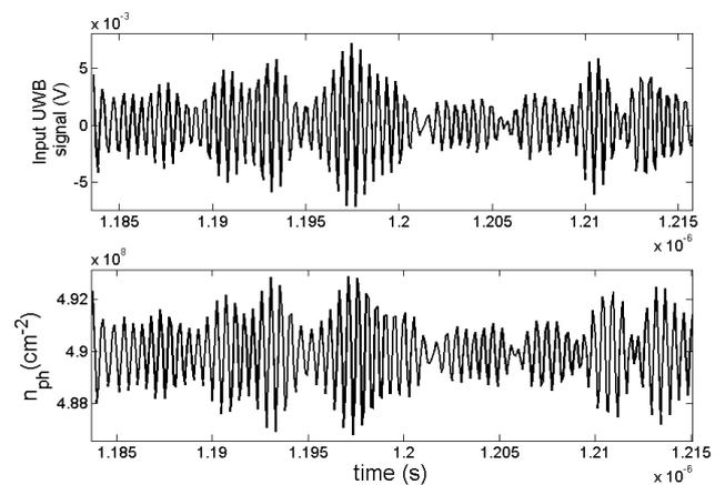
Fig. 3. The input UWB signal (upper box) and the directly modulated photon density  $n_{ph}$  (lower box)
