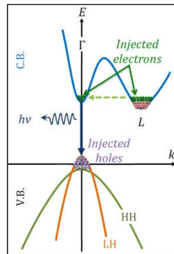
Fig. 1. Schematic diagram of the bandstructure of doped, tensile strained Ge, indicating how heavy n-type doping enhances electron injection into the  $\Gamma$  valley and hence increases the interband gain.
