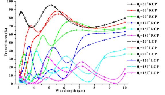
Fig. 3. Normal-incident transmittance of the TSRMMs with different groove angle  $\theta_2$ .
