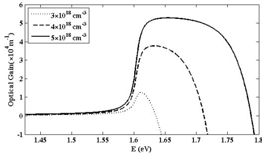
Figure1. TE mode optical gain for the three different carrier density.
