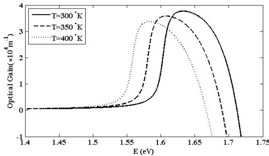
Figure2. Variation of the optical gain versus the photon energy for three different temperature.
