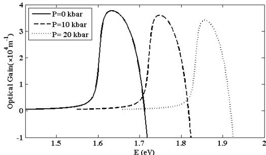
Figure3. The dependence of the optical gain on pressure in AlGaAs/GaAs DSPQW laser.
