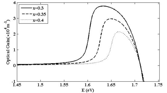
Figure4. TE mode optical gain as a function photon energy for the three different Al concentration.
