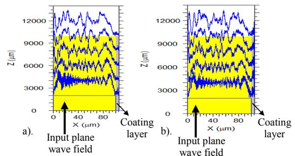
Fig. 2. a). The electric field distributions in the X-Z section as  $n_o=1.426$ ; b).The electric field distributions in the X-Z section as  $n_o=1.49$
