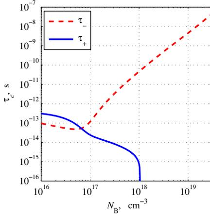
Fig. 2. Electron capture times through the phononic modes  $\omega_+, \omega_-$  for  $L_W = 3$  nm.
