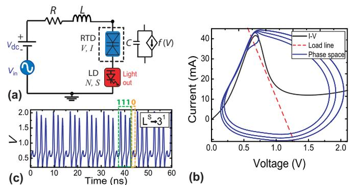
Fig. 1. (a) Equivalent circuit schematic. (b) Nonlinear I-V curve,  $f(V)$ , load line, and simulated limit cycle of a  $3^1$  MMO pattern. (c) A typical time series of a simulated  $3^1$  MMO periodic pattern.
