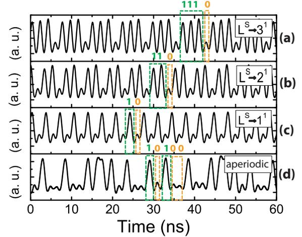
Fig. 2. (a) Experimental time traces of periodic and aperiodic MMOs for a periodic signal with an amplitude of 281 mV as a function of the injected frequency: (a) 0.544 GHz, (b) 0.564 GHz, (c) 0.586 GHz, and (d) 0.581 GHz.
