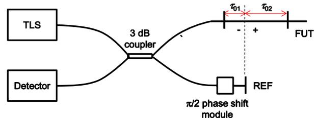
Fig. 1. Schematics of the proposed coherent OFDR system.  $\pi/2$  phase shift module is installed in the reference path. Two local reflectors are assumed to be located at both sides of reference position. TLS: tunable laser source, FUT: fiber under test
