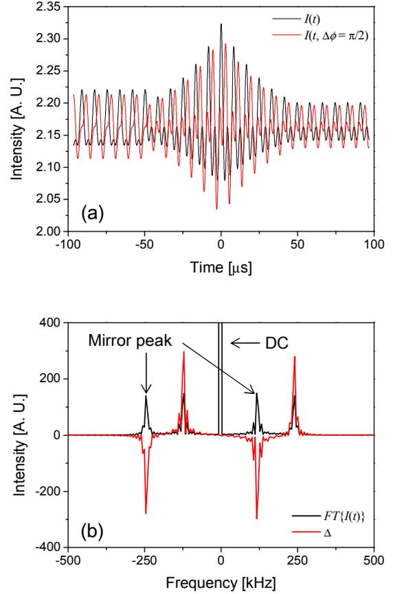
Fig. 2. (a) The original and phase-shifted signal at time-sampled photo detector obtained from the model of Fig. 1 and (b) the FFT signal with and without applying signal processing algorithm. After processing, it was obviously shown that the DC and mirror peak are eliminated.
