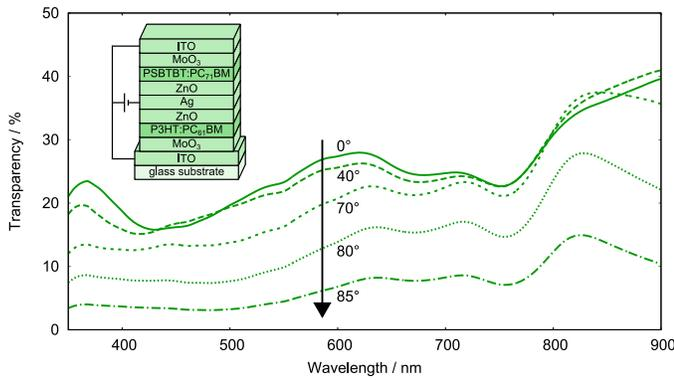
Figure 1. Spectral transparency of the tandem solar cell versus the angle of incidence of the incoming light. The inset shows a schematic representation of the simulated device architecture.
