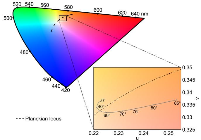
Figure 2. Chromaticities of the tandem solar cell in the CIE 1960 UCS color space versus the angle of incidence of the incoming light. In the lower part of the figure, an enlargement of the relevant part is shown.
