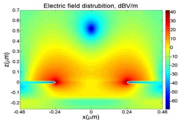
Figure 5. Electric field in cross-sectional plane in the vicinity of circular hole array.
