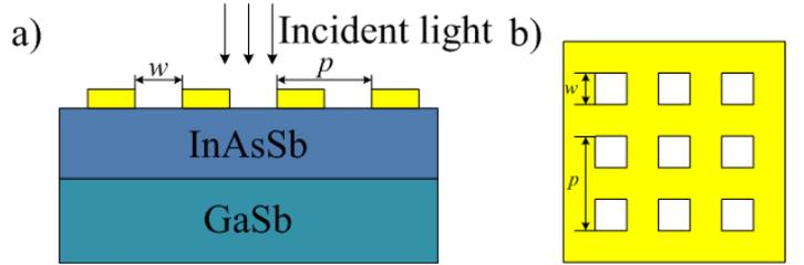
Figure 1. (a) Cross-sectional view of integrated structure. (b) Top view of hole array.
