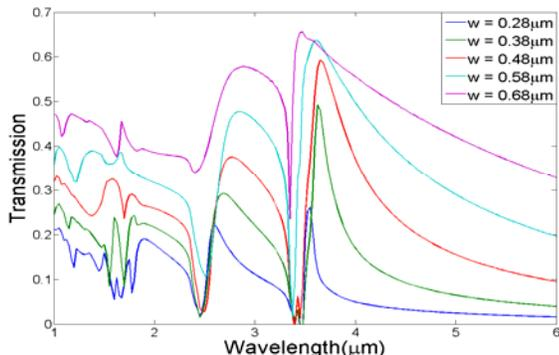
Figure 3. Simulated transmission spectrum through metallic hole array of different hole width. The hole width is varied between 0.28-0.68  $\mu\text{m}$ ,  $w = 0.48 \mu\text{m}$ ,  $t = 20 \text{ nm}$ .
