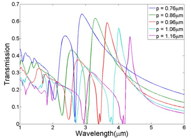
Figure 2. Simulated transmission spectrum through metallic hole array of different periodicities. The periodicity is varied between 0.76-1.16  $\mu\text{m}$ ,  $w = 0.48 \mu\text{m}$ ,  $t = 20 \text{ nm}$ .
