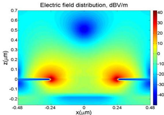
Figure 4. Electric field in cross-sectional plane in the vicinity of square hole array.
