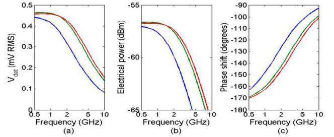
Fig. 3. Phase shifter (a) RMS detected voltage, (b) electrical power into  $50\Omega$  impedance matched load and (c) Phase shift. Blue, green and red lines are for 50 mA, 75 mA and 100 mA currents respectively. The input optical power and modulation index are -3 dBm and 5% respectively.
