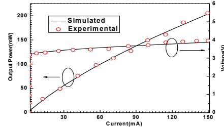
Fig. 1. Experimental and Simulated *I-V* curves and *L-I* curves of the conventional LED
