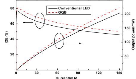
Fig. 5. IQE and light output power as a function of current for the two LED structures under study.
