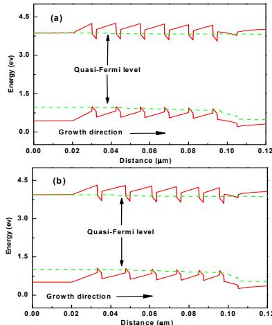
Fig. 2. (a) Energy band diagram of the conventional LED at 150mA (b) Energy band diagram of the GQB LED at 150mA
