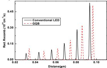
Fig. 4. Radiative recombination rate for the two LED structures at 150mA
