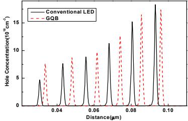
Fig.3. Hole concentrations of the two LED structures at 150mA
