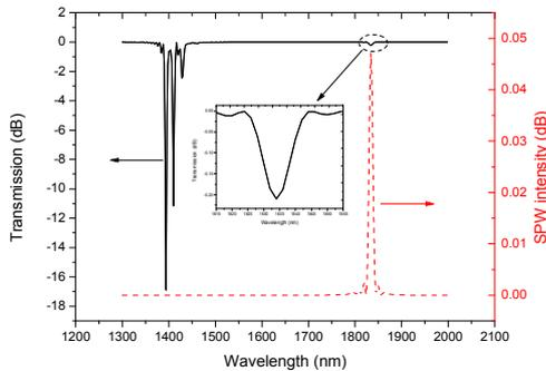
Fig. 1 Transmission and SPW intensity of a triple-clad LPFG coated with gold film
