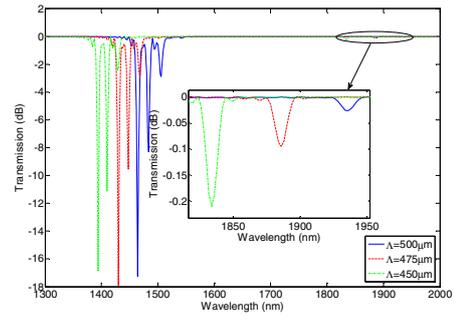
Fig. 2 Transmission spectra of LPFG coated with gold film when the grating periods are different
