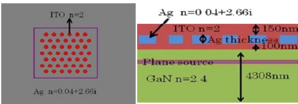
Fig. 3 Schematic illustration of the MPC inside the ITO layer.
