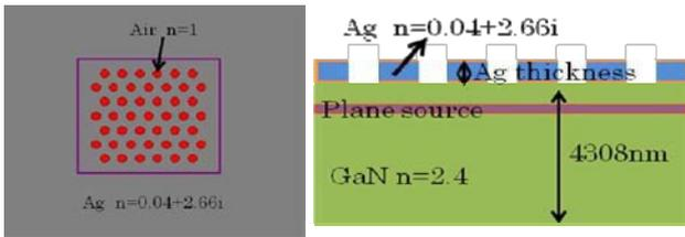
Fig. 1 Schematic of triangle array and sample cross section.
