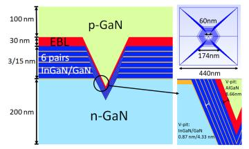
Fig. 1. Geometry of the simulation structure.
