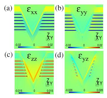
Fig. 2. Cross sectional view along the V-pit center of different strain (a)  $\epsilon_{xx}$  on the yz-plane, (b)  $\epsilon_{yy}$  on the yz-plane, (c)  $\epsilon_{zz}$  on the yz-plane, and (d)  $\epsilon_{yz}$  on the yz-plane.
