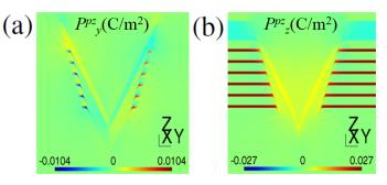
Fig. 3. Cross sectional view along the V-pit center of different piezoelectric polarization direction (a) piezoelectric polarization along y-axis on the yz-plane, and (b) piezoelectric polarization along z-axis on the yz-plane.
