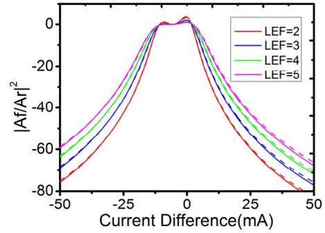
Fig.4 The difference of amplitude ratio  $|A_i/A_r|^2$  caused by different LEF, the same color indicates the same LEF, the dash curve of each color is  $PDR = 2 \times 10^9 s^{-1}$ , when the solid curve  $PDR = 0$
