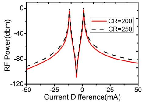
Fig.5 The output RF power curve with different coupling rate (CR), and  $PDR = 2 \times 10^9 s^{-1}$ .
