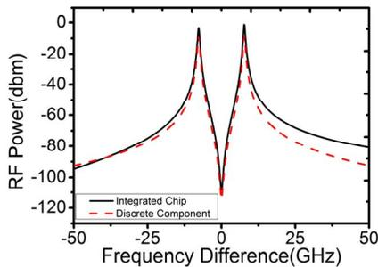
Fig.2 Output RF Power curve of two section DFB laser (asymmetric) and two discrete lasers (symmetric)
