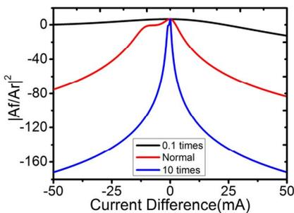
Fig.3 The difference of amplitude ratio  $|A_i/A_r|^2$  caused by the wavelength change rate (nm/mA)
