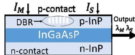
Fig.1 The structure of the two section DFB laser
