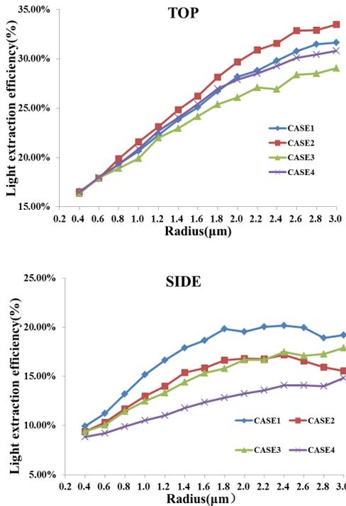
Fig. 4. LEE from top and four side facets of PSS-LED chip as a function of radius, when the distance is  $7\mu\text{m}$
