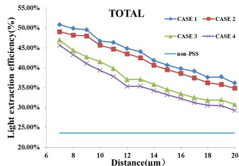
Fig. 2. LEE of the LED flip chip with hemispherical patterns on the two surfaces of the sapphire substrate.
