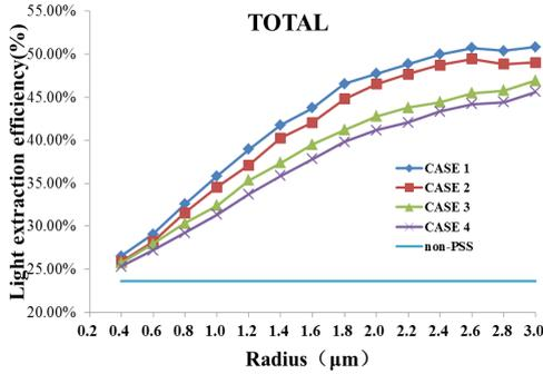
Fig. 3. Total LEE of flip chips grown on hemispherical PSS with optimized distance as a function of the radius
