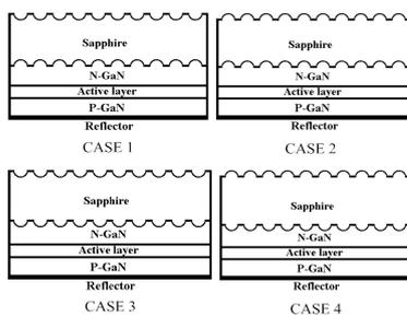
Fig. 1. Four types of hemispherical pattern on the two surfaces of the sapphire substrate.
