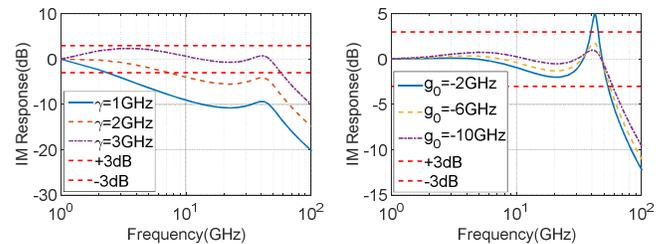
Fig. 2. The impact of parameters  $\gamma$  and  $|g_0|$  on the IM response. Left: increase  $\gamma$  while keeping  $g_0=-10\text{GHz}$ ,  $f_{CRP}=10\text{GHz}$ ,  $f_{PPR}=40\text{GHz}$ ; Right: increase  $|g_0|$  while keeping  $\gamma=6\text{GHz}$ ,  $f_{CRP}=10\text{GHz}$ ,  $f_{PPR}=40\text{GHz}$ .
