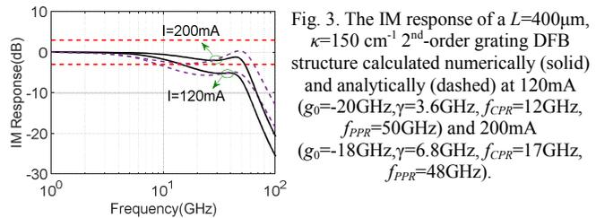
Fig. 3. The IM response of a  $L=400\mu\text{m}$ ,  $\kappa=150\text{ cm}^{-1}$  2<sup>nd</sup>-order grating DFB structure calculated numerically (solid) and analytically (dashed) at 120mA ( $g_0=-20\text{GHz}$ ,  $\gamma=3.6\text{GHz}$ ,  $f_{CRP}=12\text{GHz}$ ,  $f_{PPR}=50\text{GHz}$ ) and 200mA ( $g_0=-18\text{GHz}$ ,  $\gamma=6.8\text{GHz}$ ,  $f_{CRP}=17\text{GHz}$ ,  $f_{PPR}=48\text{GHz}$ ).
