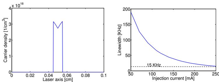
Fig. 3. Carrier density profile and spectral linewidth of the optimized laser with anti-reflection facets and  $\lambda/4$  phase shift at the center of resonant cavity
