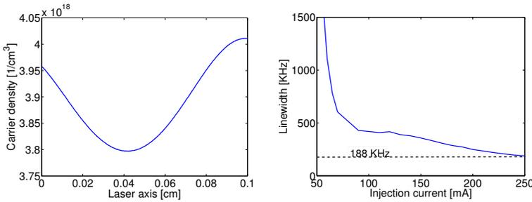
Fig. 2. Carrier density profile and spectral linewidth of the standard DFB laser with cleaved facets and  $\lambda/4$  phase shift at left facet
