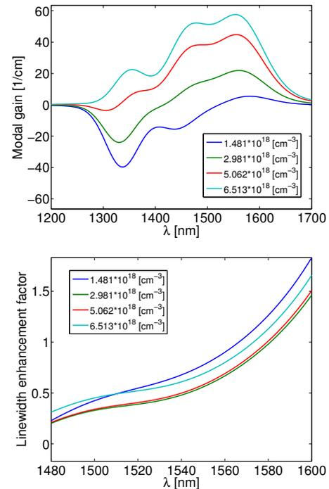
Fig. 1. Calculated dispersion of modal gain and linewidth enhancement factor of a  $1.55\mu\text{m}$  multiple QD-layer epi-structure
