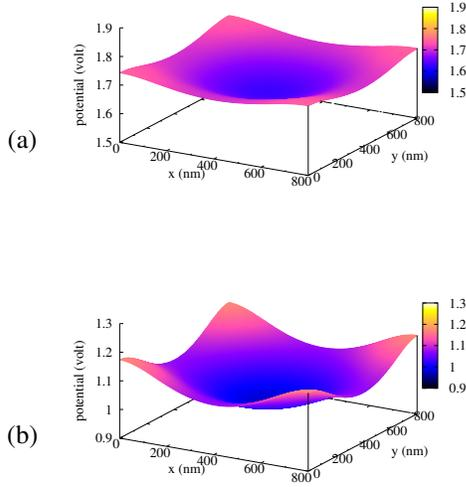
Fig. 2. (a) Spatial distributions of electric potential along the active region within the UC (a) Realistic case of the mesh strips with square cross-section  $100 \times 100 \text{ nm}^2$ ; (b) Analytical model based on thick-wire approximation for the mesh strips. Mesh pitch  $a = 800 \text{ nm}$ , applied bias voltage  $V = 2.5 \text{ V}$ .
