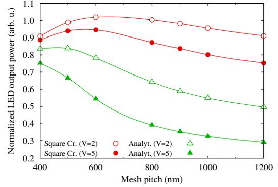
Fig. 3. Normalized total output optical power versus mesh pitch  $a$ , calculated for (a) mesh strips with square cross-section  $100 \times 100 \text{ nm}^2$  and (b) analytical approximation of mesh strips as wires of finite radius.
