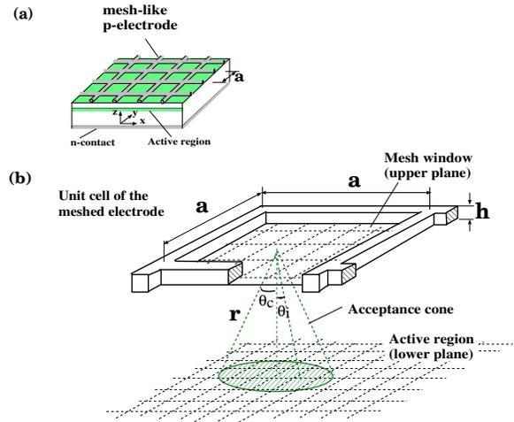
Fig. 1. (a) Schematics of the LED with top p-electrode designed as a mesh. (b) Bi-plane computation domain for the LED's unit cell. Strips of the meshed electrode have square cross-section. Lower and upper planes correspond to a light-generating layer and output semiconductor-air interface, respectively.
