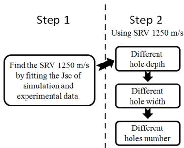
Fig. 1 The diagram of two-step simulation flow chart.
