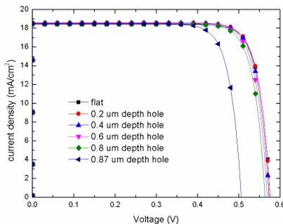
Fig. 2 The simulated photovoltaic J-V curves as a function of the hole depth based on the SRV of 1250 m/s.
