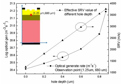
Fig. 3 The simulated optical generate rate and SRV as a function of the hole depth based on the SRV of 1250 m/s.
