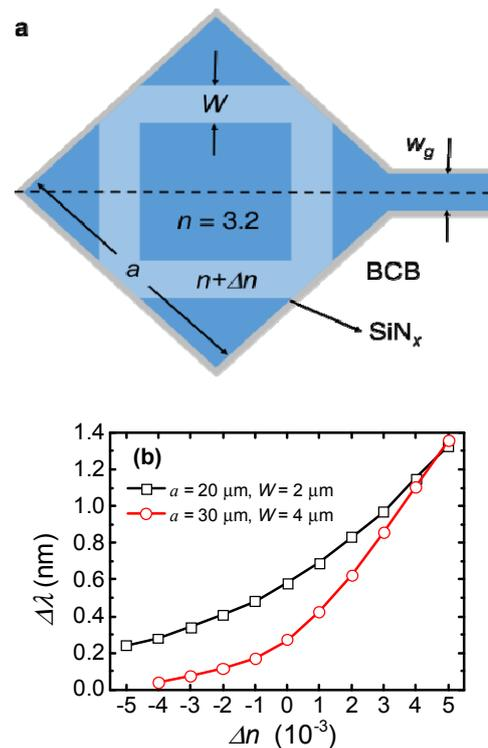
Fig. 1. (a) Schematic of the square microlaser with a square-ring electrode, and (b) the simulated mode wavelength intervals versus  $\Delta n$  for the square resonators with the side length  $a = 20 \mu\text{m}$ ,  $w_g = 1.5 \mu\text{m}$ ,  $W = 2 \mu\text{m}$  (square symbols), and  $a = 30 \mu\text{m}$ ,  $w_g = 2.5 \mu\text{m}$ ,  $W = 4 \mu\text{m}$  (circular symbols), respectively.
