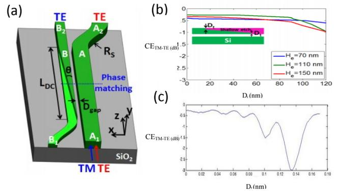
Fig.4. (a)Schematic of the PSR based on the taper-etched directional coupler, (b) Dependence of the polarization conversion efficiency to tip width  $D_t$ , sweeping from 0 to 120 nm reported by Xiong[2], (c) Investigation on dependence of the polarization conversion efficiency to tip width  $D_t$ , sweeping from 0 to 180 nm
