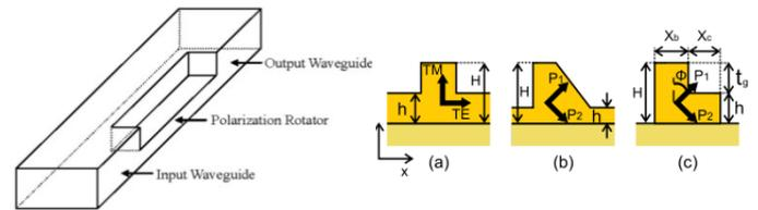
Fig.1. The stepped waveguide polarization rotator presented by Wang [3] (left), Transverse geometries of (a) interconnection waveguide, (b) slanted waveguide rotator, (c) stepped waveguide rotator. [1]
