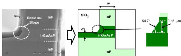
Fig.3. SEM result for the etching profile (left) and cross-sectional model based on actual structure of the fabricated device (right) [4]
