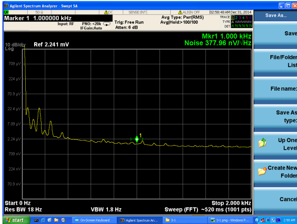
Fig. 3. Measured noise spectrum of the epitaxial Si:P BIB detector enclosed by liquid helium at anode bias of 3V.
