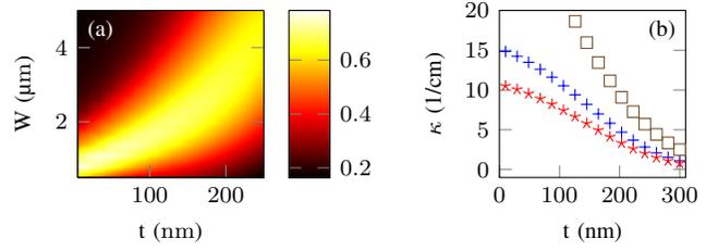
Fig. 2. Variation of (a)  $\Gamma_{123}^\pm$  as a function of ridge width and etching depth and (b)  $\kappa$  as a function of unetched cladding thickness evaluated using (5) (+), (6) and convolution (\*), and (6) with  $n_{\text{eff}}$  values for wide and narrow ridge slices obtained directly from a MS ( $\square$ ).
