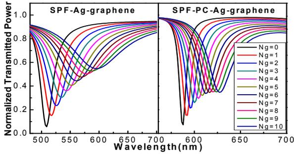
**Fig.3.** (Left) The normalized transmitted power spectra of SPF-Ag-graphene and (Right) SPF-PC-Ag-graphene for the RI of 1.333 for the surrounding area where the number of graphene layers ranging from 0 to 10.
