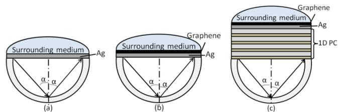
Fig. 2. Schematic diagram of (a) SPF-Ag, (b) SPF-Ag-graphene, and (c) SPF-PC-Ag-graphene configurations.
