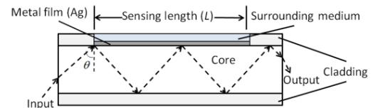
Fig. 1. The meridional cross section of SPR sensor based on side polished fiber
