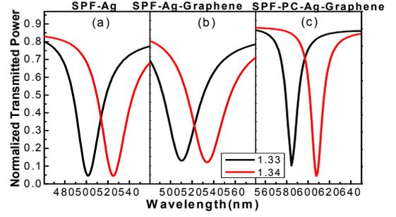
**Fig. 4.** The normalized transmitted power spectra of (a) SPF-Ag, (b) SPF-Ag-graphene and (c) SPF-PC-Ag-graphene configuration respectively while the RI of the surrounding medium are 1.33 and 1.34.
