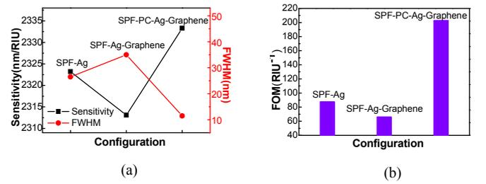
**Fig. 5.** (a) is The sensitivity and FWHM in SPF-Ag, SPF-Ag-graphene, and SPF-PC-Ag-graphene configurations respectively. (b) is the FOM in SPF-Ag, SPF-Ag-graphene, and SPF-PC-Ag-graphene configurations respectively.
