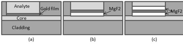
Fig. 1. The physical models of CSPR (a), LRSPR (b) and SSPR (c).
