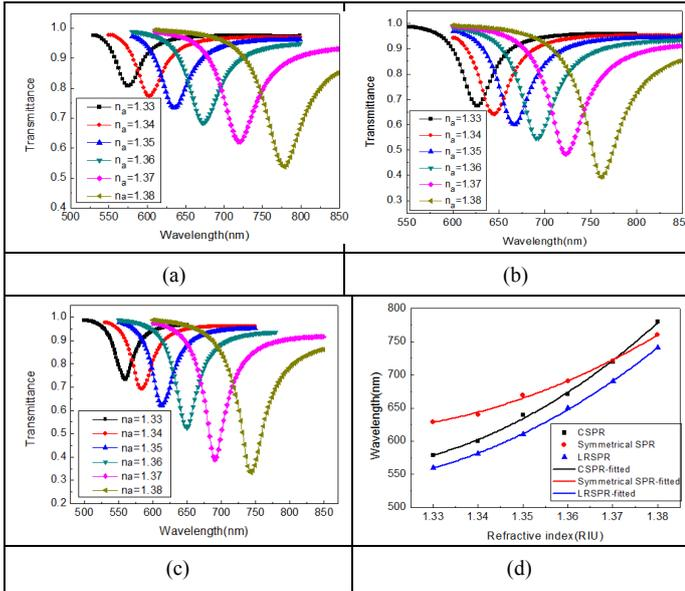
Fig. 2. The resonance spectra for CSPR (a), SSPR (b) and LRSPR (c). The dependence of resonance wavelength on the refractive index (d).
