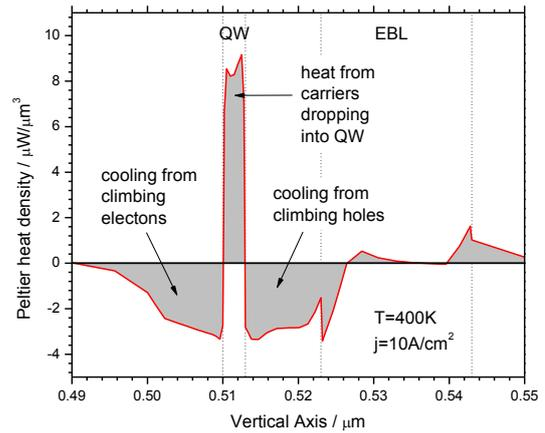
Fig. 3: Vertical Peltier heat profiles near the quantum well.
