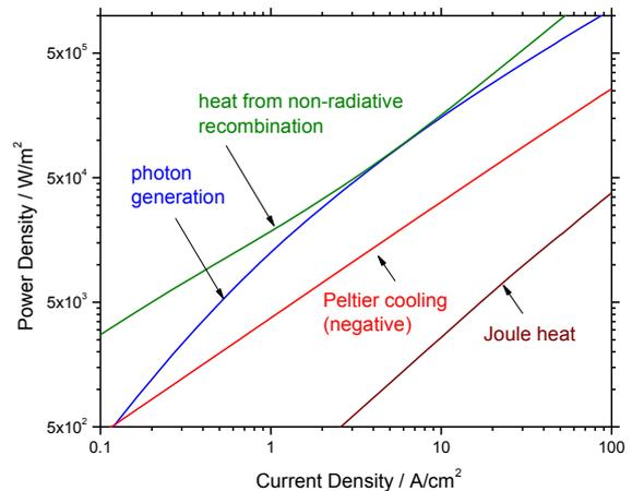
Fig. 4: Contributions to the total LED power budget vs. current.
