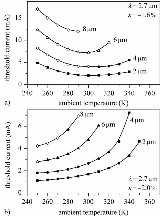
Fig. 3. Calculated threshold current vs. ambient temperature for 2.7- $\mu\text{m}$  VCSEL with a) 1.6% and b) 2.0% compressively strained QWs. Filled and empty symbols correspond to  $\text{LP}_{01}$  and  $\text{LP}_{11}$  mode operation, respectively.
