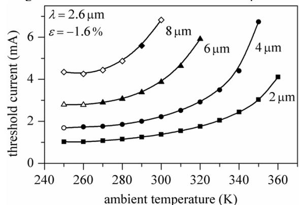
Fig. 1. Calculated threshold current vs. ambient temperature for 2.6- $\mu\text{m}$  VCSEL with 1.6% compressively strained QWs. Filled and empty symbols correspond to  $\text{LP}_{01}$  and  $\text{LP}_{11}$  mode operation, respectively.
