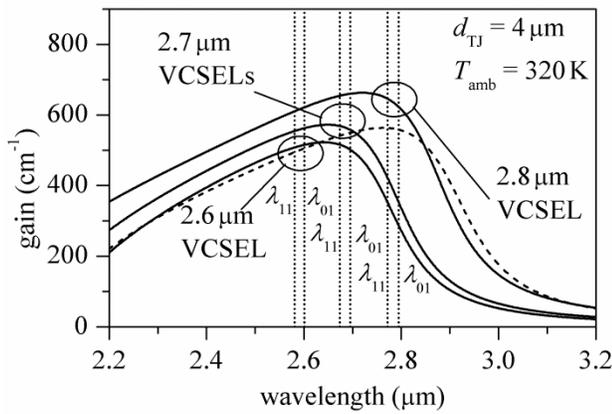
Fig. 2. Gain spectra calculated for VCSELs with 4- $\mu\text{m}$  TJ diameter emitting in the 2.6–2.8  $\mu\text{m}$  wavelength range with 1.6% (solid lines) and 2.0% (dashed line) compressively strained QWs. Wavelengths corresponding to the  $\text{LP}_{01}$  and  $\text{LP}_{11}$  modes have been additionally shown.
