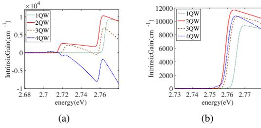
Fig. 2: The gain curve of different quantum well numbers structure. 2(a) All the structures' gain does not rise at the same energy level due to different screen of QCSE. 2(b) After adjust the indium composition, the gain rise at the same energy level.
