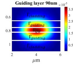
Fig. 4: The optical confinement  $\Gamma$  for different areas
