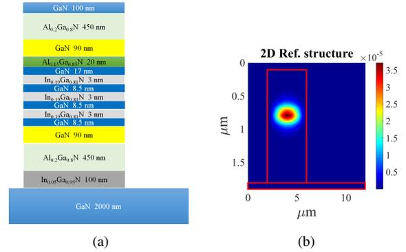
Fig. 1: (a) the laser diode structure in the simulation. (b) is the cavity mode of 2D optical field of the LD structure.
