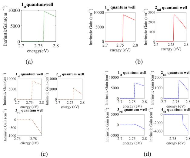
Fig. 3: (a), (b), (c), and (d) are the gain curves in each QW of the 1,2,3 and 4 quantum wells structure. The gain of each single QW is plot separately to investigate the reason of the negative gain.
