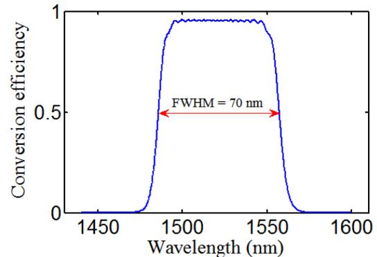
Fig. 3 Numerical results for conversion efficiency from x-polarized mode at the input to z-polarized mode at the output vs. input wavelength
