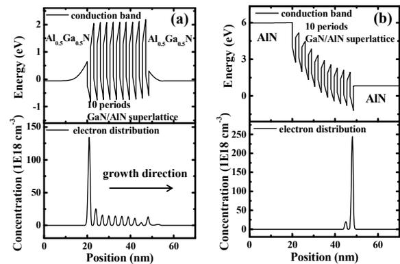
Fig. 1 Conduction band profile and electron distribution for a ten periods GaN/AlN superlattice sandwiched between  $\text{Al}_{0.5}\text{Ga}_{0.5}\text{N}$  and AlN claddings.
