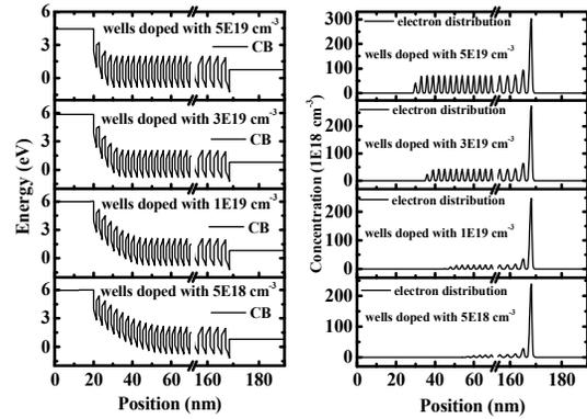
Fig. 3 Conduction band profile and electron distribution with different doping concentrations in wells.
