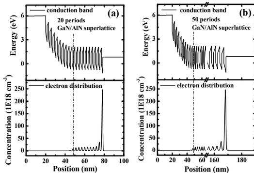
Fig. 2 Conduction band profile and electron distribution for a twenty periods and a fifty periods GaN/AlN superlattices.
