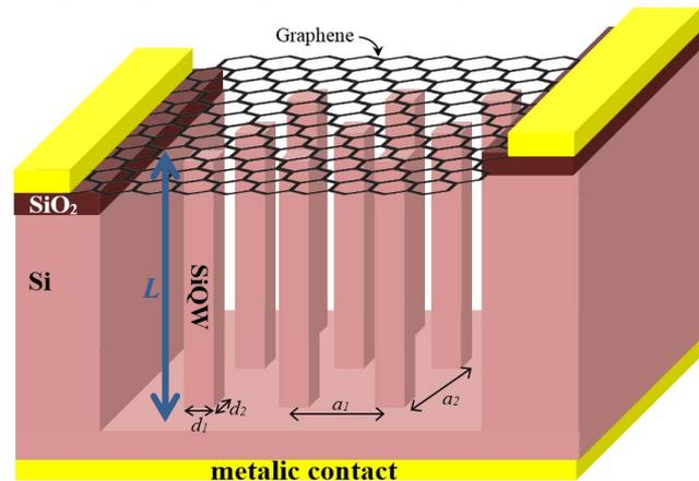
Fig. 1: Schematic view of the SiQWs/G solar cell.
