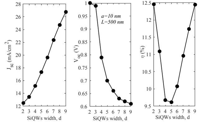
Fig. 3:  $J_{sc}$ ,  $V_{oc}$  and  $\eta$  of p-SiQWs/G solar cells as functions of SiQWs width.
