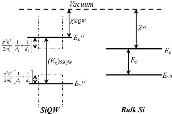
Fig. 3. A band diagram of a SiQW and bulk Si.  $\chi_{Si}$ ,  $E_g$ ,  $E_{c0}$  and  $E_{v0}$  correspond to the electron affinity, band gap, conduction and valence band edge of Si, respectively.  $\chi_{SiNW}$ ,  $(E_g)_{SiNW}$ ,  $E_{c}^{II}$  and  $E_{v}^{II}$  correspond to the electron affinity, band gap, first conduction and valence subband edge of SiQW, respectively.
