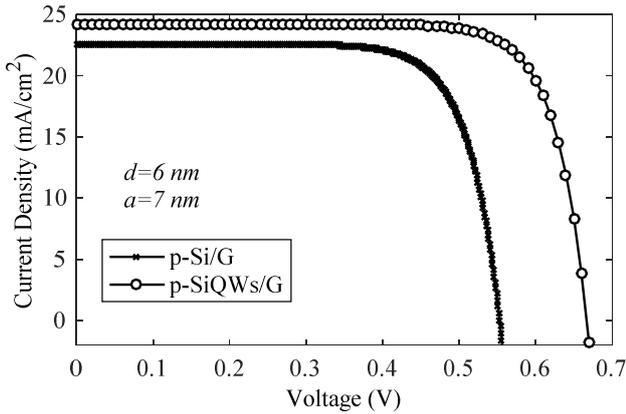
Fig. 2: photo-current density–voltage characteristics of p-type Si/G and SiQWs/G solar cells.
