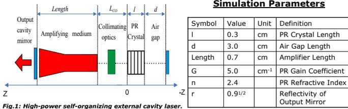
Fig. 1: High-power self-organizing external cavity laser.
