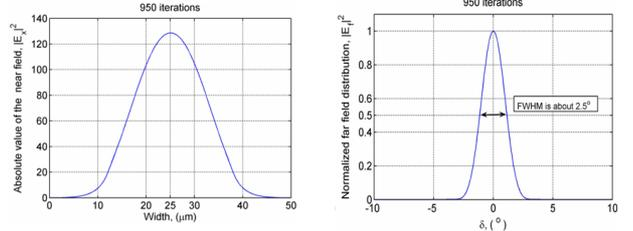
Fig. 4: The distribution of the near-field (left) and the far-field (right).
