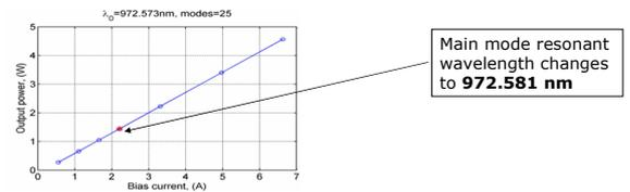
Fig. 6: The light-current characteristics of the main mode.
