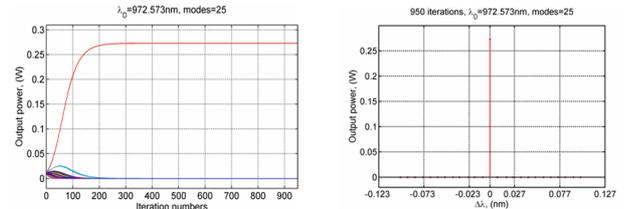
Fig. 3: The iteration procedure of the resonant modes (left); The converged output power for every mode (right).
