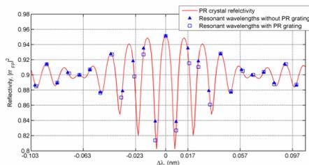
Fig. 2: Comparison of the reflectivity of the resonant modes and possible modes.
