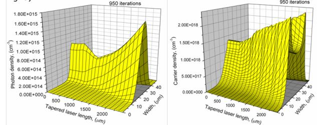
Fig. 5: The 2D photon density distribution of the main mode (left) and the carrier density (right).
