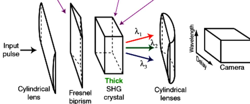
A *single* optic (a Fresnel biprism) replaces the *entire* delay line, and a *thick* SHG crystal replaces *both* the thin crystal *and* spectrometer.
